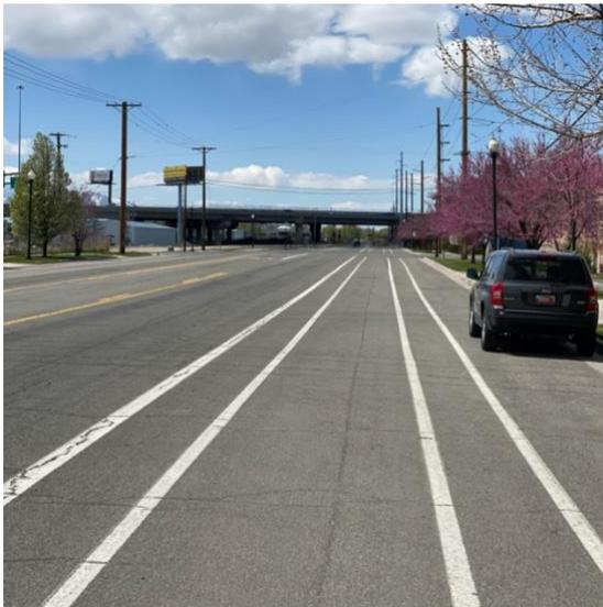
*Figure 2: A view of 900 South at 450 West showing clearly marked bicycle lanes that reduce conflict between vehicles and cyclists.*
